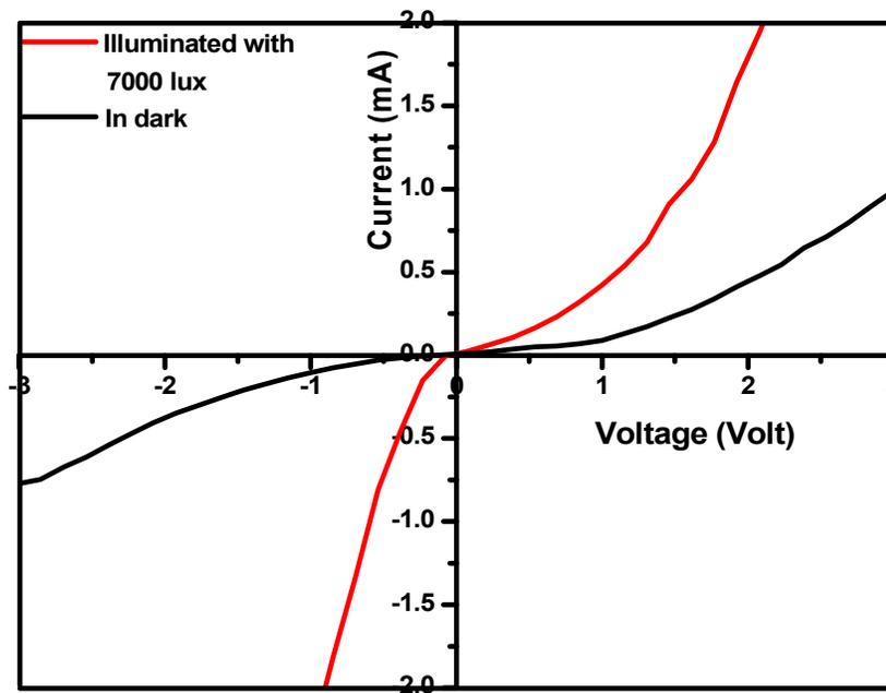
**Fig. No. 9 I-V Characteristic in dark and illumination at 7000 lux light intensity for n-CdSe/p-Cu<sub>2</sub>S thin film .**
