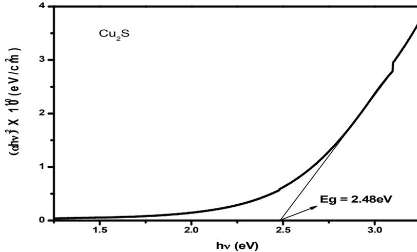
**Fig. No. 7 Optical energy band gap of Cu<sub>2</sub>S thin films**
