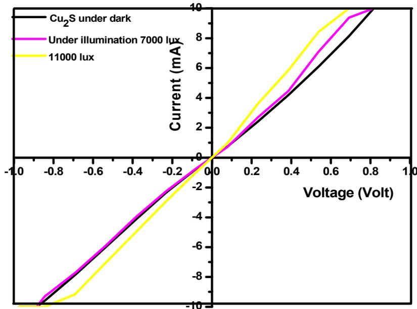
**Fig. No. 8 I-V Characteristic of  $\text{Cu}_2\text{S}$  thin film in dark and under illumination.**
