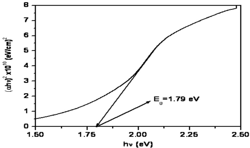
Fig. No. 4 Optical energy band gap of CdSe thin films
