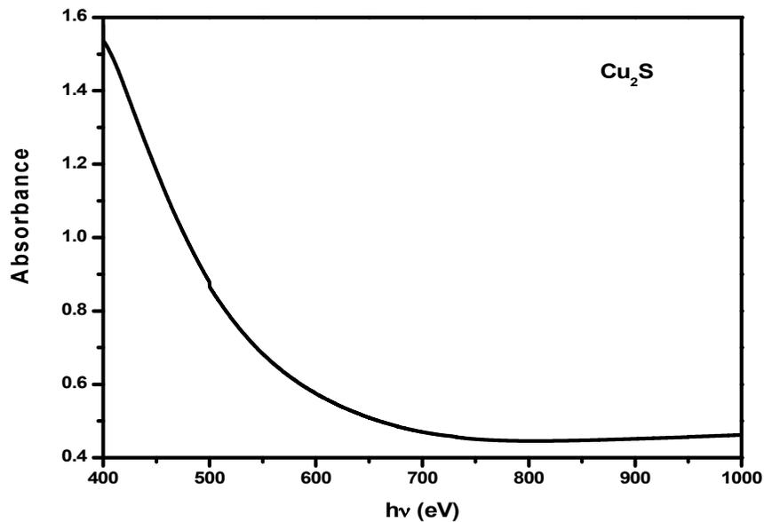
**Fig. No. 6 Absorbance of as-deposited Cu<sub>2</sub>S thin film.**
