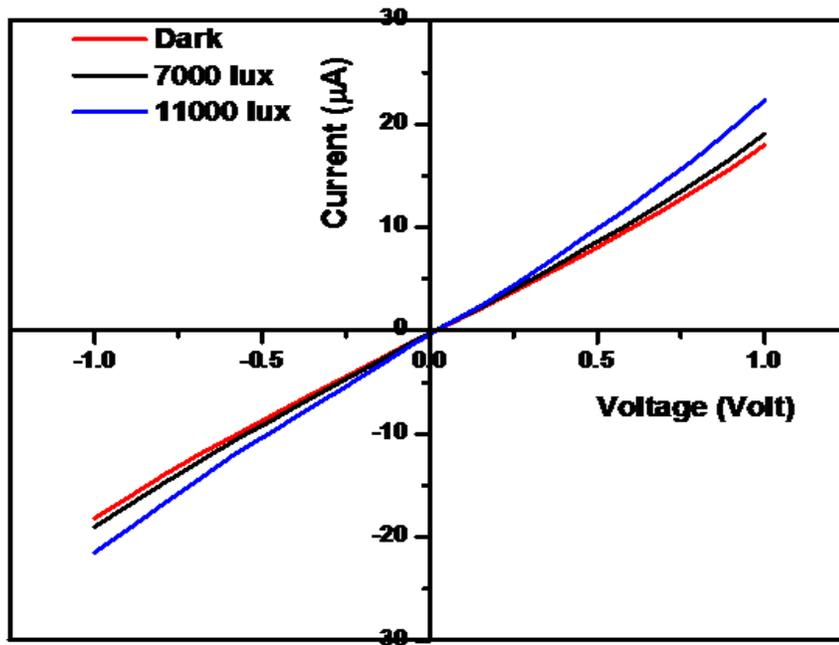
Fig. No. 5 I-V Characteristic of CdSe thin film in dark and under illumination.
