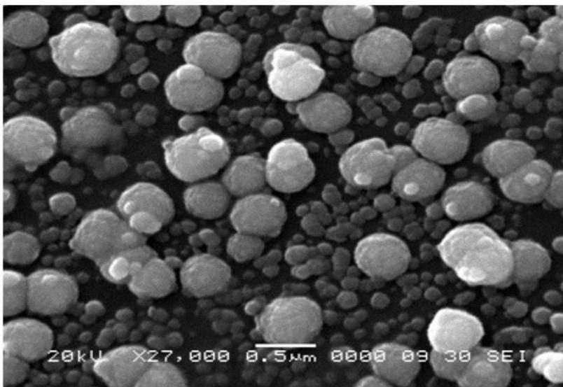
**Fig. No. 2 SEM image of as-deposited CdSe thin film.**
