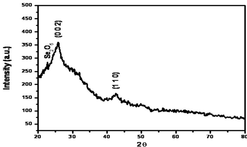
Fig. No.1 X-ray diffraction pattern of as –deposited CdSe thin film.
